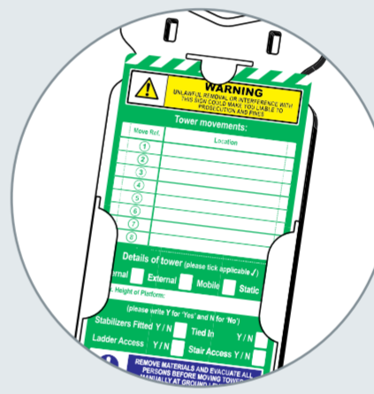
Tower relocation record
